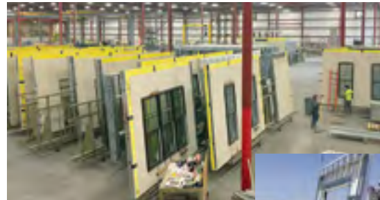
Panelized exterior wall assemblies reduce labor requirements up to 50%
